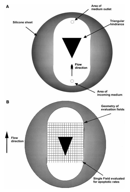
**FIG. 1.** Geometry of the perfusion area. (A) The geometry of the chamber's flow zone and the placement of the triangular hindrance are shown. (B) The arrangement and size of the single fields evaluated for apoptotic rates are shown.
