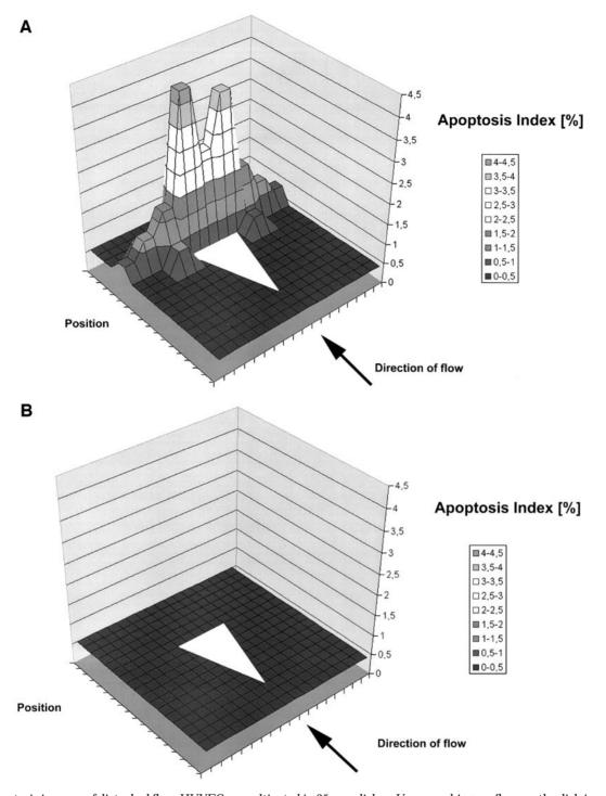
**FIG. 2.** Apoptosis in areas of disturbed flow. HUVEC are cultivated in 35-mm dishes. Upon reaching confluence, the dish is converted into a perfusion chamber and cultivation continued with a mean shear stress of 5 dyn cm $^{-2}$  (calculated for the chamber without hindrance) for an additional 3 days. Apoptotic rates (expressed as a percentage) for cell populations of individual areas are determined and plotted as bars. A was without and B was with addition of anti-receptor antibodies.
